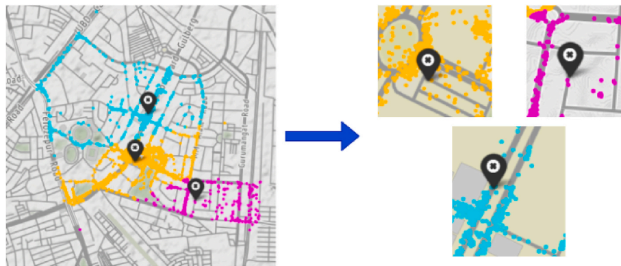
Fig. 7. Visualization of the substations that are projected to the nearest point that corresponds to a road so that finally we could have on-road placement of substations.
